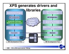
Now once we have the model for our system implementation, there is one more step. We have generate all the necessary drivers for the peripherals that we installed and we also have to generate the libraries that we've selected.
