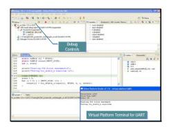
This is the perspective for the debugger. Again, we mentioned that the perspective changes depending on what your task is within the tool. We happen to be in the debugging perspective and in the upper-left window, you'll see above that window a variety of different debug options. I can run, I can stop, I can single-step, I can step into and out of functions -- again, all of the normal things I would expect from a debugger. These are standard features within Eclipse.
