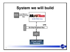
Now, if we want to build a system, we have to decide what we're going to build. For, today, we've got a limited amount of time, so we're going to build a very simple system. We're going to instantiate MicroBlaze. We're going to give it a local memory, and we're also going to instantiate a UART or an RS232 or giving us a terminal to view printf() results out of our software program.
