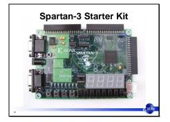
For those of you who are might be interesting in the Spartan family, this is a soft core so you can target a Spartan board as well. As we mentioned, soft cores can target any of the devices available from Xilinx -either the Virtex or the Spartan family. So this would be a low cost, about \$100 Starter Kit board that you could use for experiments.
