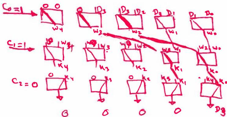
There is  $\log_2 n = 3$  rows of muxes so the delay of 3 shifts = delay of 5 shifts =  $3 \tau_m$
