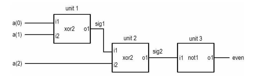
Even detector using previously designed components (xor2 and not1)
