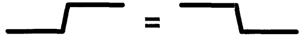
FIGURE 2. Two Equivalent Transitions Rising and falling transitions on signalling wires have the same meaning. They are called events.
