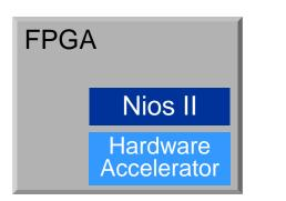
Add external coprocessing hardware to accelerate data functions Multiprocessor System
